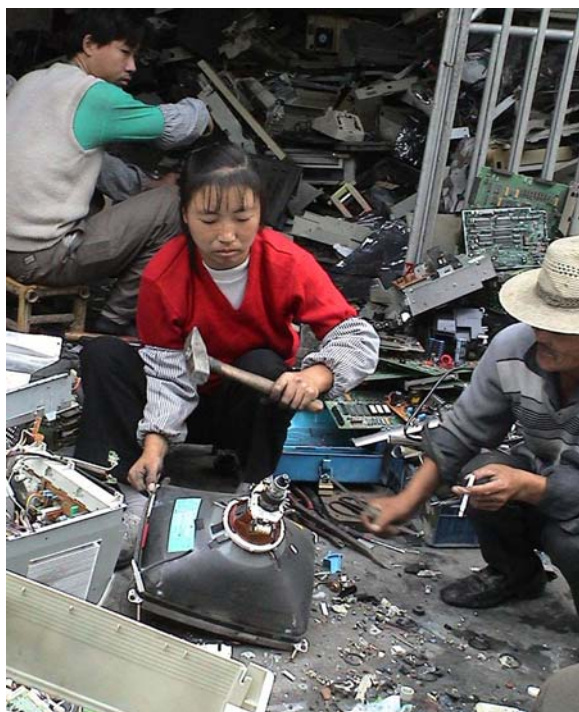
Woman in Guiyu, China, about to smash a cathode ray tube from a computer monitor, to remove the copper yoke at the end of the funnel. The glass is laden with lead, but the biggest hazard from this is the inhalation of the highly toxic phosphor dust coating inside of the CRT. © Basel Action Network 2001
